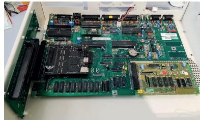
ABOVE: Picture of Zorro board and A500 board in tray and screw locations
