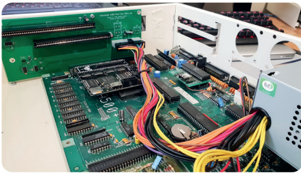
ABOVE: Zorro board with power cable connected.
